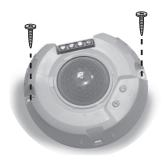
C. Access to terminal blocks, screws and potentiometer: To get access to the above mentioned items, simply remove the front cover.
