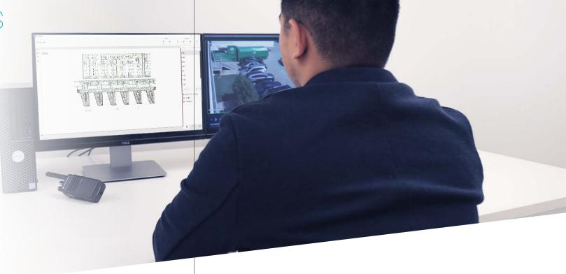
Normalink BMS allows the monitoring from any computer connected to the same local network as the rest of Normalink devices (gateways with DALI luminaires, addressable central battery systems with 24 Vdc emergency lights, inputs-outputs modules, etc.). It is also possible to monitor remotely through Normalink Cloud.
